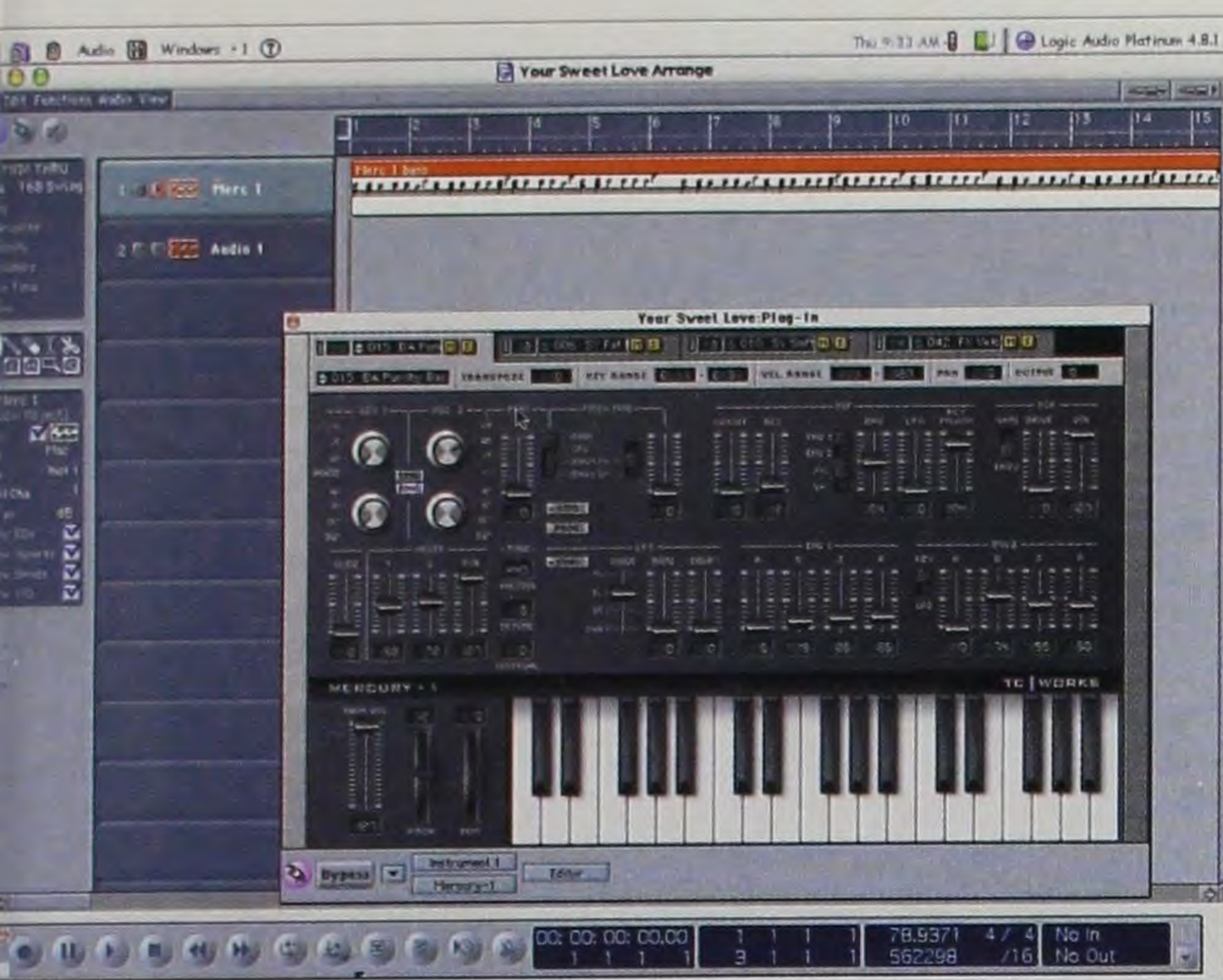
Figure 2 The TC Works Mercury-1 softsynth. It can emulate classic analog subtractive synthesizers.
