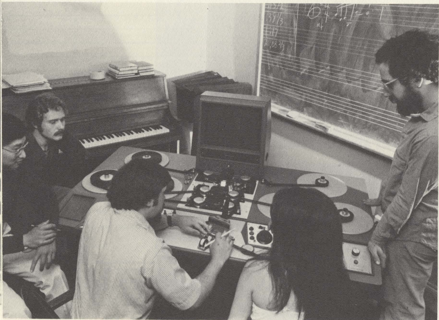
Don Wilkins, Chairman of the Berklee Film Scoring Department, demonstrates the use of "Moviola" in synchronizing dialogue and video with musical sound track
